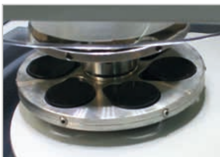
Central pressure requires levelled samples
