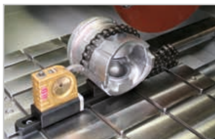
Guide bar with chain clamping vice
