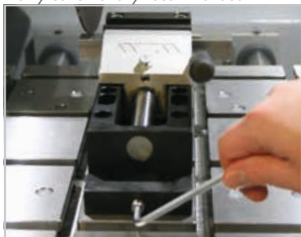
Change of preassembled Easy-clamping bases
