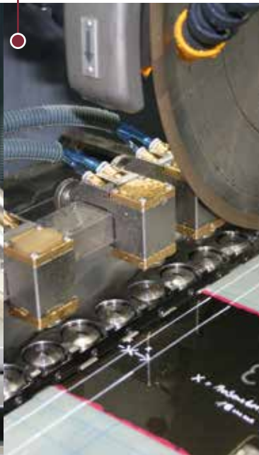
Pulsed clamping system for automatic parallel cutting of GFK and CFK plates
