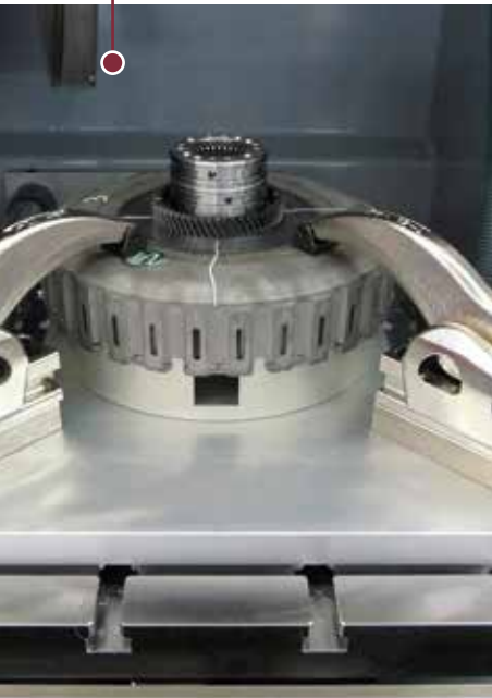
Special clamping device for clutch case
