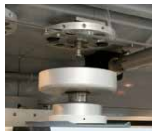
Automatic feed from sample holder magazine
